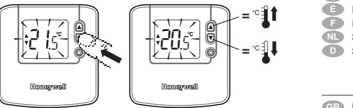
**GB** Switch ON/OFF (frost protection enabled)
